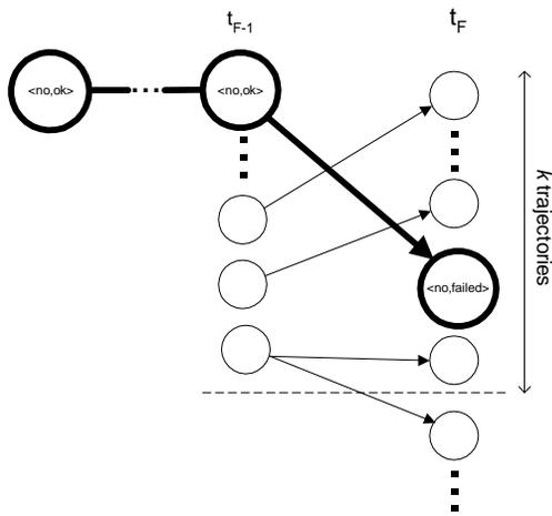
Figure 3: Failure detection with  $k$ -best enumeration. In this figure, the trajectories are shown ordered in terms of their posterior probability, with the most likely at the top. Trajectories below the dashed line are discarded. The mode trajectory is shown in bold.
