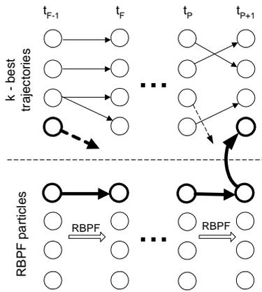
Figure 5: Failure detection with our mixed method. At time  $t_F$  the true trajectory (bold line) is no longer among the trajectories with the  $k$  highest posteriors. However, the true trajectory is sampled stochastically and becomes a member of the RBPf particle set. At time  $t_{P+1}$ , the posterior of the true trajectory becomes large enough for it to be included in the leading  $k$  trajectories.
