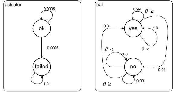
Figure 2: Discrete transition model for an acrobatic robot. If the actuator has failed, it exerts no torque. When the robot catches the ball,  $\text{ball}=\text{yes}$ , and the mass of the lower link increases.
